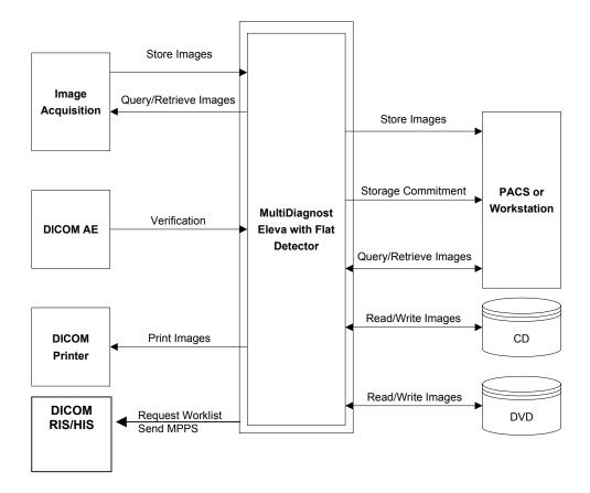
Figure 1: MultiDiagnost Eleva with Flat Detector System in a DICOM Network environment
